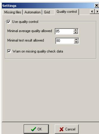
The **Quality control** tab accommodates settings, related to playlist media files, which have been passed through quality control tests. Such tests are performed by the **QCBox** tool. For more detailed information, related to **QCBox**, please, refer to the relevant chapter further in this manual.
