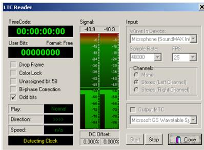
If you are licensed to use the **LTC reader** module and you have a *DirectSound* compatible sound card, you may use it to read LTC timecode from your transport device. The setup of this module is quite simple. Select your sound card device from the list. Select *Sample rate* and *Channels* and **Start** the module. The current timecode is shown in the *TC Timer*.
