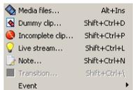
Both commands provide the same action list. The difference is in the insertion point in the playlist. While an **Add** command will add the selected event at the end of the playlist, the **Insert** command will insert the selected event above the currently selected line.
