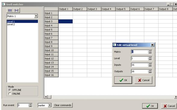
This optional plugin is used to control Snell devices that comply with the SW -P-08 protocol. It uses RS-485 cables. COM port settings may vary for different devices. The matrix is configured in the same way as the Sierra Video Switcher event's one above. The only difference is that here you can set more than one matrix, in case you have more than one device.
