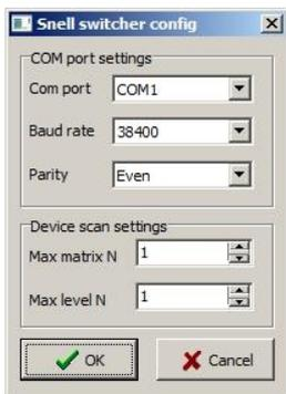
This is an external plug-in used to control Snell devices that comply with the *SW-P-08* protocol. It uses *RS-485* cables. The COM port settings may vary for different devices.
