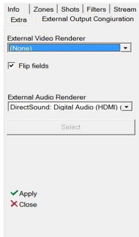
In this tab you can select an *External Video Renderer*, as well as an *External Audio Renderer* from the drop-down lists. For the video renderer you are able to flip the fields of the output video by checking the *Flip fields* box.
