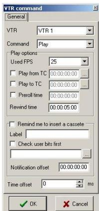
Although **AirBox** was designed as a file-based playout engine, now you can control up to 2 external VTRs through *RS422* for tape-based playout. All you have to do is insert a VTR control event in the playlist.
